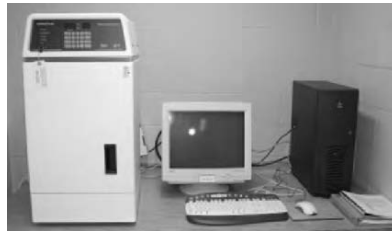
Figure 5-11. Faxitron digital X-ray machine used at the Ornamental Plant Germplasm Center.
