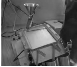
Figure 5-10. Small single deck vibrating table used at the Ornamental Plant Germplasm Center.
