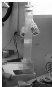
Figure 5-9. Single column seed blower used at the Ornamental Plant Germplasm Center.
