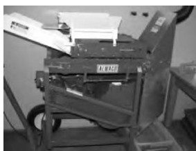
Figure 5-8. Modified small seed-lot belt thresher, showing the blocking of the original built-in winnowing component by a chute that direct the threshed seed and chaff down to a screened container at the Ornamental Plant Germplasm Center.
