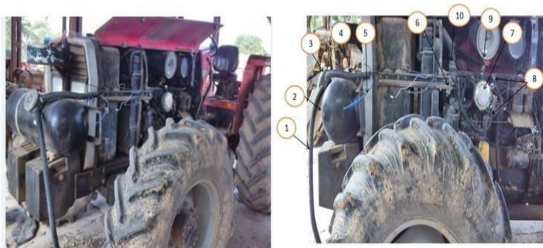
Figure 1 and 2 – how synthetic fuel system of gasoline and LPG is implemented on a MF399 tractor
